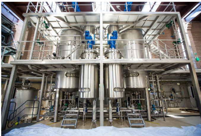
56 Pilot scale state-of-the-art 1.5 m 3 and 15 m 3 fermentation equipment for industrial bioprocessing at BBEPP.
